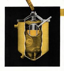
Oil can't drain back to the crankcase and give you a false oil-level reading... if you have an AC "5-Star Quality" Oil Filter. When the engine stops the oil stays right where it belongs, because of the high position of the outlet. And the outlet can't clog, because only clean oil passes through it.
